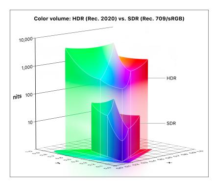
HDR displays typically process video at 10 bits per color component rather than 8 bits. The additional color data lets HDR displays render more discrete steps from the minimum to maximum brightness value in each color.
