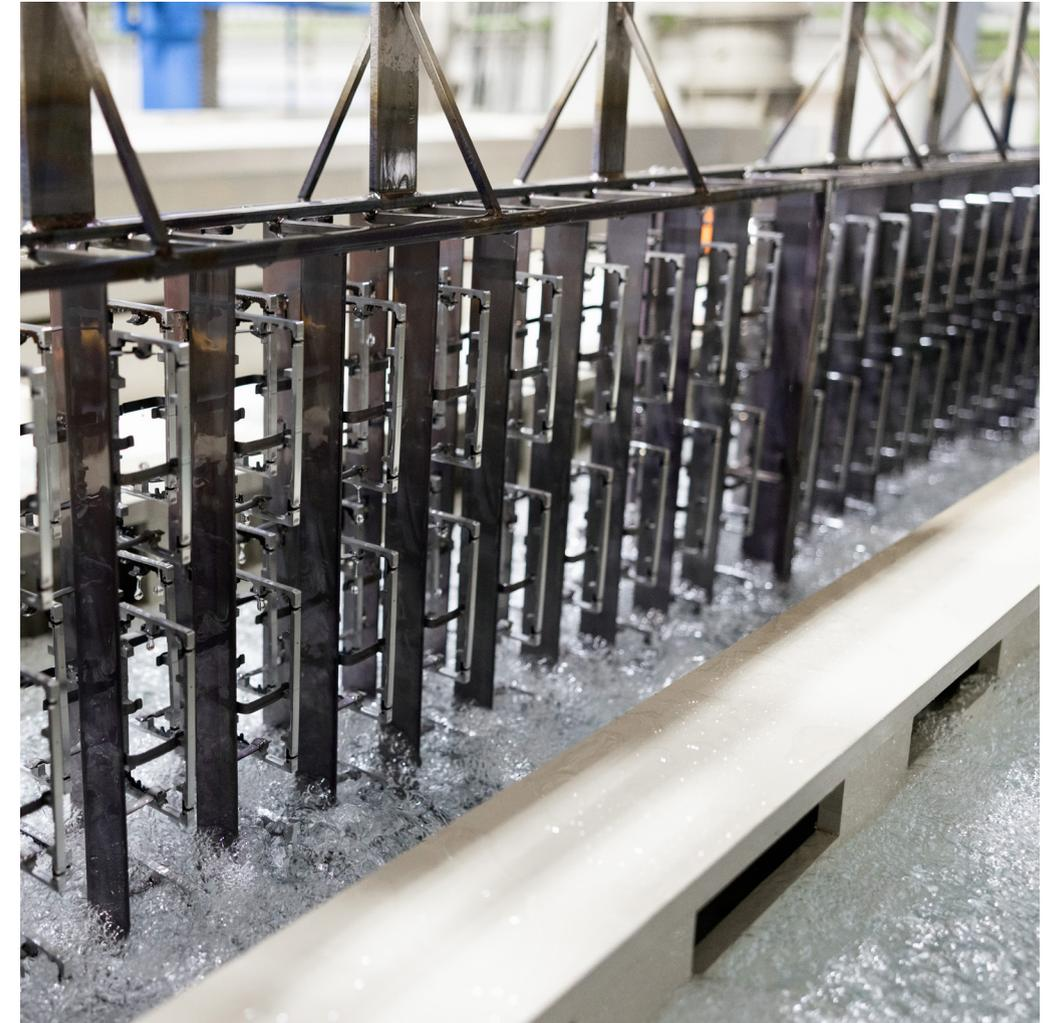
We continued our initiative focusing on enhancing and supporting our electrochemical metal-finishing processes, like anodizing, which has the potential to save hundreds of millions of gallons of water annually when applied at scale.
