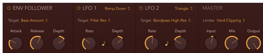
Changes by modulator parameters are reflected by blue rings and dots around target parameter knobs, making it easy to identify a target parameter that is being modulated. The rings indicate the range (modulation depth) and the dots indicate the current value of the modulator. Realtime, manual XY pad modulation is also indicated in a similar way for target parameters.
