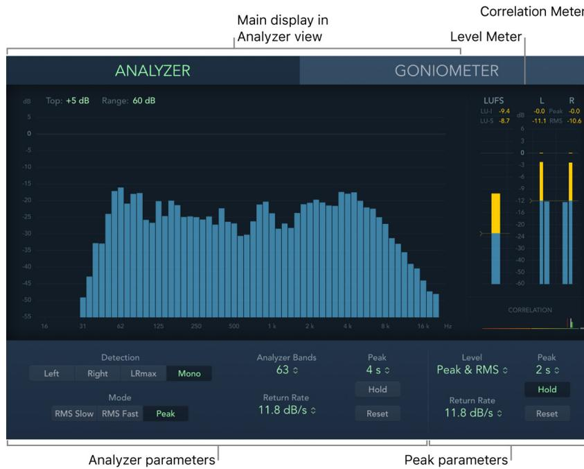
Although you can insert MultiMeter directly into any channel strip, it is more commonly used in the master channel strip of Logic Pro—when you are working on the overall mix.
