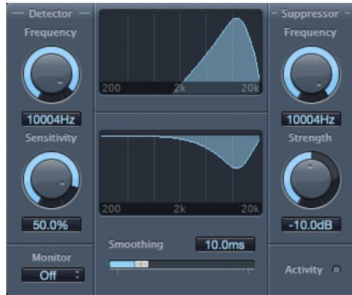
The Detector parameters are on the left and the Suppressor parameters are on the right. The center section includes the Detector and Suppressor displays and the Smoothing slider.
