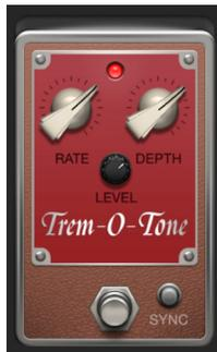
Trem-O-Tone is a simple tremolo effect—modulation of the signal level.
