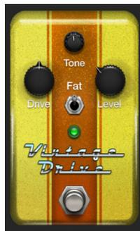
Vintage Drive is an overdrive effect that emulates the distortion produced by a field-effect transistor (FET), commonly used in solid-state amplifiers. When saturated, FETs generate a warmer-sounding distortion than bipolar transistors, such as those emulated by Grinder.
