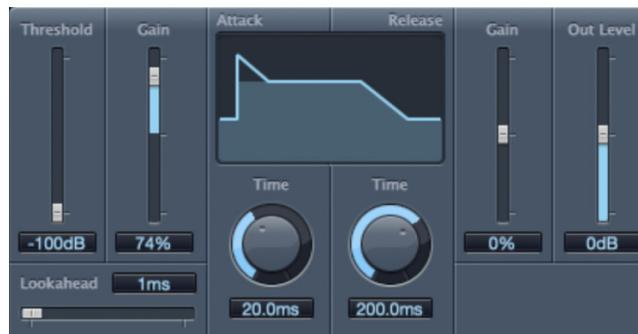
The most important Enveloper parameters are the two Gain sliders, one on each side of the central display. These govern the Attack and Release levels of each respective phase.
