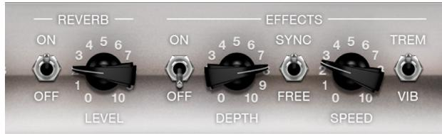
Reverb, which is controlled by an On/Off switch in the middle, can be added to either tremolo or vibrato, or it can be used independently. See [Amp Designer reverb effect](#).
