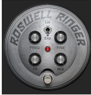
Roswell Ringer is a ring modulation effect that can make incoming audio sound metallic or unrecognizable, and can deliver tremolos, brighten up signals, and more. See [Ringshifter overview](#) for information on ring modulation.
